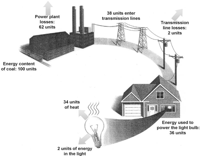
Figure 1-2 Energy Losses in Powering a Light Bulb
